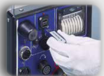
USB memory stick for saving, loading and archiving of welding programs and monitored welding data
