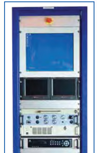
Perfect traceability when combining video together with real-time welding parameter monitoring and recording
