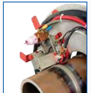
Quick change of the electrode
