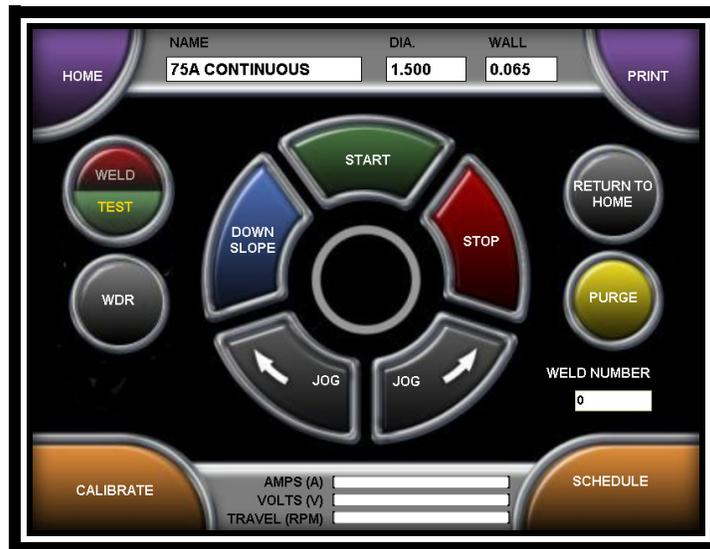
8. Press START to initiate the weld. The center of the RUN screen displays a count-down of each weld sequence.
