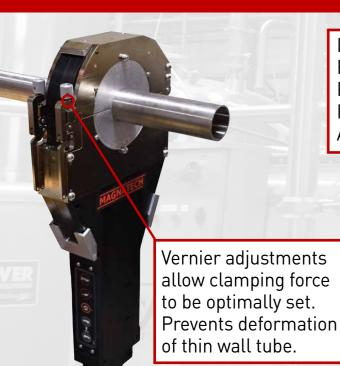
Indestructible Nickel Reinforced Hinge Provides Rigidity For Positive Tube Alignment.
