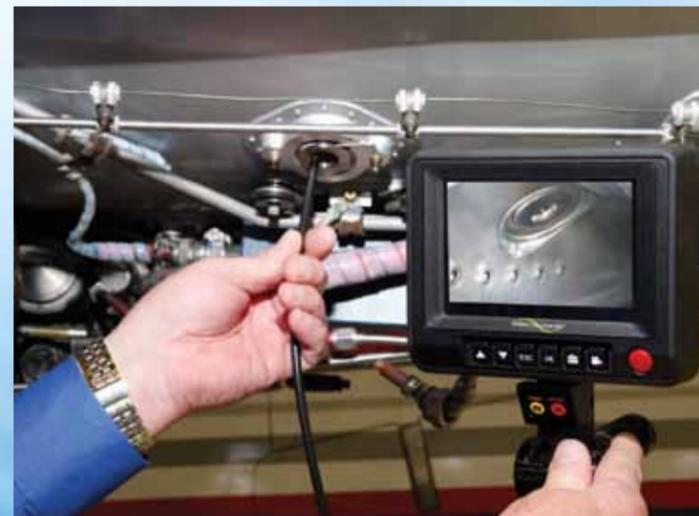
Aircraft and Power Generation maintenance teams can quickly and easily inspect turbine blades, combustion chambers, cooling tubes, and much more, all without the need for costly and time consuming engine and system tear-down. Foundries can inspect for flash, sand, and voids inside complex castings.
