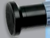
Hawkeye<sup>®</sup> Blue Swing Prism Borescopes have a tiny prism at the tip that pivots, or "swings," to vary the direction-of-view from 16° to 118°. A ring on the borescope body controls the prism direction. The fieldof-view is 45°, so the borescope effectively sees from -7° to 133°.
