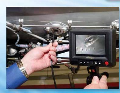
Aircraft and Power Generation maintenance teams can quickly and easily inspect turbine blades, combustion chambers, cooling tubes, and much more, all without the need for costly and time consuming engine and system tear-down. Foundries can inspect for flash, sand, and voids inside complex castings.
