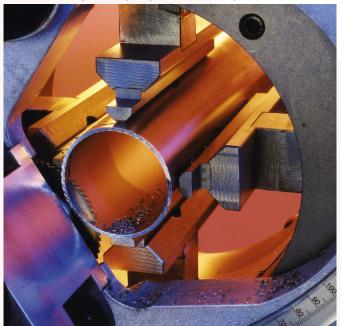
The precision of our cutting machine allow a perfect tube to tube alignement, with the smallest gap possible, removing the need to facing the tube therefore saving a significant amount of time and money.
