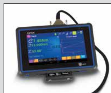
Check monitoring screen with relevant torque operation values
