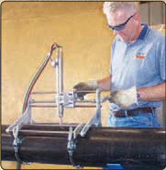
An excellent tool for making coupons for bend, tensile strength, and hardness tests.
