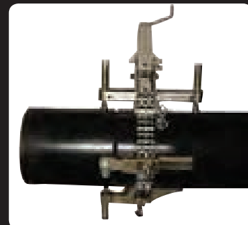
Pipe to pipe horizontal (Single Jackscrew Jackbar)
