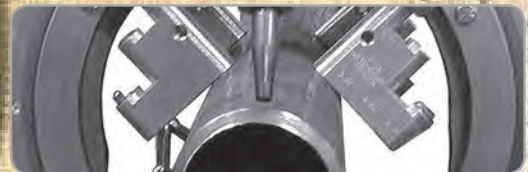
1SA Saddle Machine shown on 3" (76 mm) pipe
