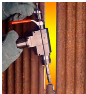
Only 1.5" wide for single boiler tube beveling
