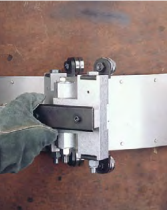
Trolley is adjustable to fit all Esco Wrap Tracks
