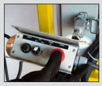
Each unit comes with a remote electrical pendant equipped with hydraulic flow and direction controls as well as an automatic shut-off button.
